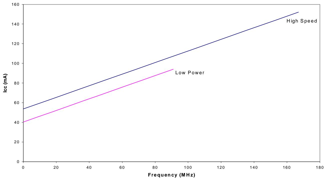
The typical pattern is a 16-bit up counter, per logic block, with outputs disabled.
