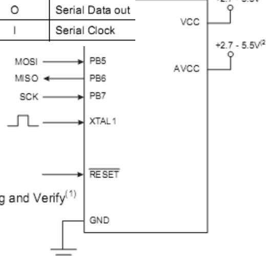
Figure 136. SPI Serial Programming and Verify<sup>(1)</sup>
