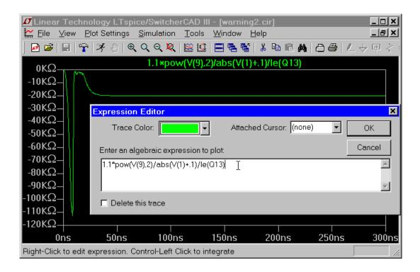
The difference of two voltages; e.g., V(a)-V(b); can equivalently written as V(a,b). The following functions are available for real data:
