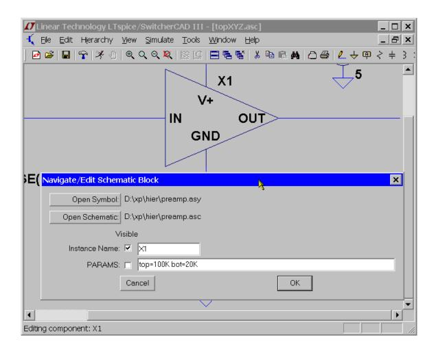
Note that is dialog also allows you to enter parameters to pass to this instance of the circuitry in preamp.asc.
