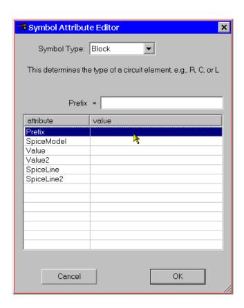
The symbol's attributes can be overridden in the instance of the symbol as a component in a schematic. For example, if you have a symbol for a MOSFET with a prefix attribute of 'M', it's possible to override the prefix to an 'X' on an instance-by-instance basis so that the transistor can be modeled as subcircuit instead.
