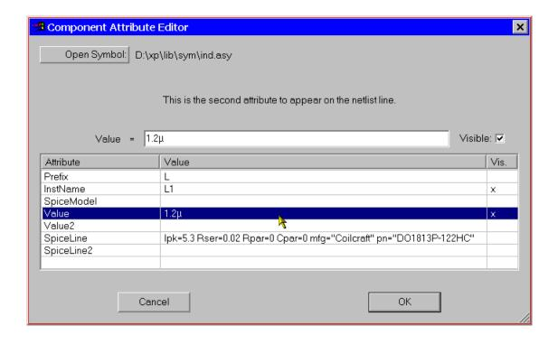
The attributes SpiceModel, Value, Value2, SpiceLine, and SpiceLine2 are all part of the overall value of the component. In terms of the way the component is netlisted for SPICE, the component will generate a line of SPICE that looks like this:
