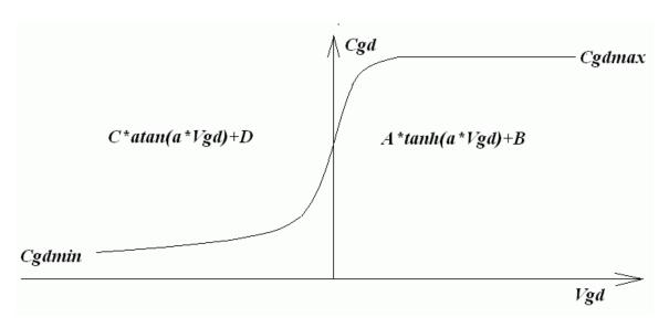
For positive Vgd, Cgd varies as the hyperbolic tangent of Vgd. For negative Vdg, Cgd varies as the arc tangent of Vgd. The model parameters a, Cgdmax, and Cgdmax parameterize the gate drain capacitance. The source-drain capacitance is supplied by the graded capacitance of a body diode connected across the source drain electrodes, outside of the source and drain resistances.
