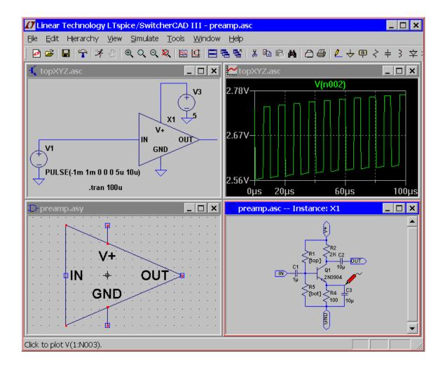
LTspice will look in the directory of the top-level schematic for symbols and blocks to complete the circuitry of the top-level schematic.
