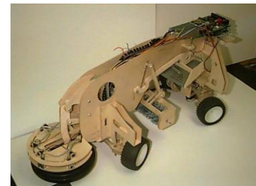
Hyena: Metal detector and collector
