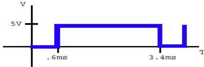
Figure 3: Period of the clock signal entering the cuecat from the PC.
