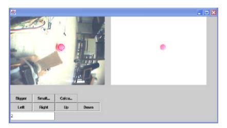
The desired object is clicked on. To more precisely vary the size and position of the circle the *Bigger, Smaller, Left, Right, Up & Down* buttons are provided. After the object is encapsulated, the user enters the number of standards deviations away from the mean that the threshold should be set at by entering the number in the textbox and then clicking on the *Calculate Histogram* button.
