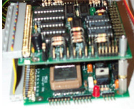
Figure 1 The MSRX01 board is on top. The MRC11 board is on the bottom. The chip in the brown socket is the 68HC11.
