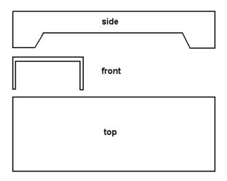
Designing the mobile platform was kind of a paradox. A stronger frame is required to hold the motor and batteries and to stand up to the large forces; but as the frame gets larger and stronger, more batteries and a larger motor are required to move it. I chose to build the platform out of plywood for its low cost and because it is easy to work with. A strong plastic would most likely provide better performance.
