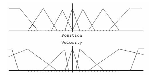
The percent power to send to the motors is determined from these two functions. The membership value in each category is then used with the table below to determine the power.
