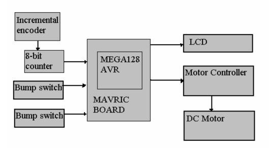
The control system has one external input, the angle of the pendulum. The output of the control system is the force Billy's motor must exert to move either forward or backwards. Past input data will be used to determine the pendulum's angular velocity. These two values are used by the control system to determine the output.
