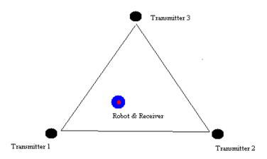
The transmitters are arbitrarily placed in a equilateral triangle, with side length of 10 feet (for now). The robot will determine the distance away from each transmitter to calculate its current coordinate. Pulses by each transmitter will triggered at fixed intervals of 0.5s, with a period of 4s, as shown below. However, 4 seconds was not practical for updating coordinate, so instead, this was changed to 2 seconds.
