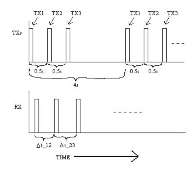
The receiver (robot) determines the time difference between each of the pulses to compute coordinate. The exact equations can be found in the Appendix.
