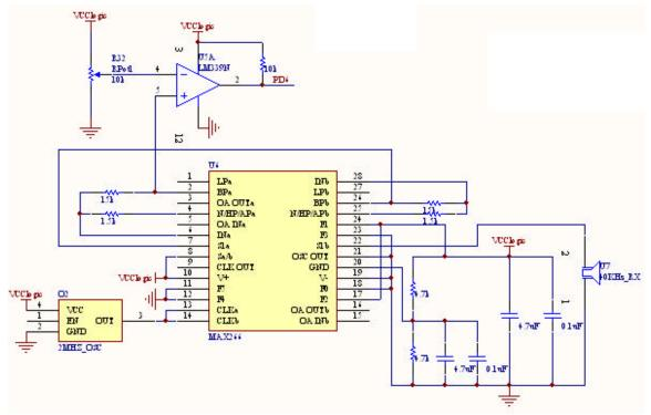
The output of this system is pin 2 of the LM339N comparator. This signal was fed directly to the input capture pin of the microcontroller.
