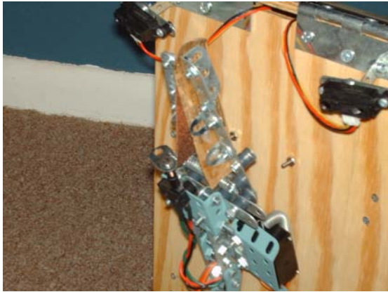
Figure 1: Front of robot showing IR sensors
