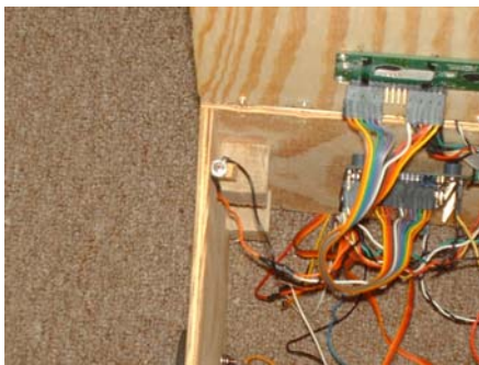
Figure 2: The bump switch located under the lid
