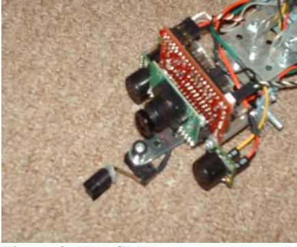
Figure 3: The CMU camera mounted under the robotic arm
