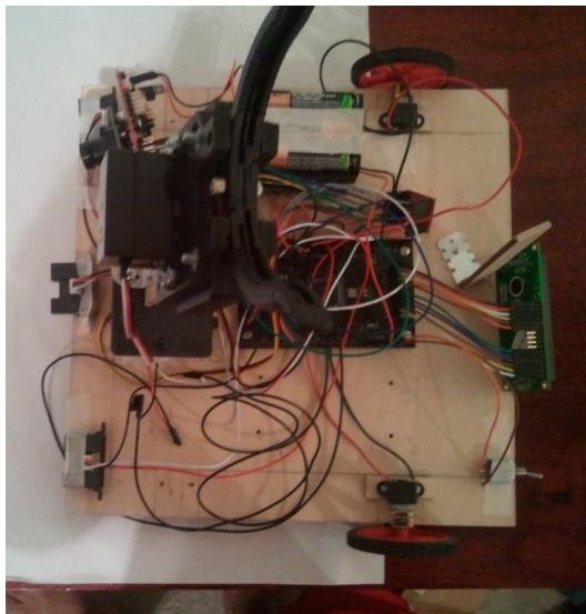
The mobile platform took a long time to be built. The gripper and the tilt drive had to be assembled and due to the inferior quality, all the parts weren't fitting smoothly. I had to use a cutting blade to modify the components so that they would fit smoothly.
