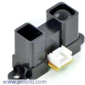
Three Sharp GP2Y0A02YK0F IR rangefinder sensors are used. Two of them are used for obstacle avoidance and one of them is used for cup detection.
