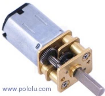
Mobile actuation was enabled using two 298:1 micro metal gear motors from Pololu. These gear motors are extremely small and so they do not take up a large footprint on the platform. They have the highest torque – lowest power ratings in their category, which met the overall goal of the robot not travelling too fast, and being able to support all the weight on the base.
