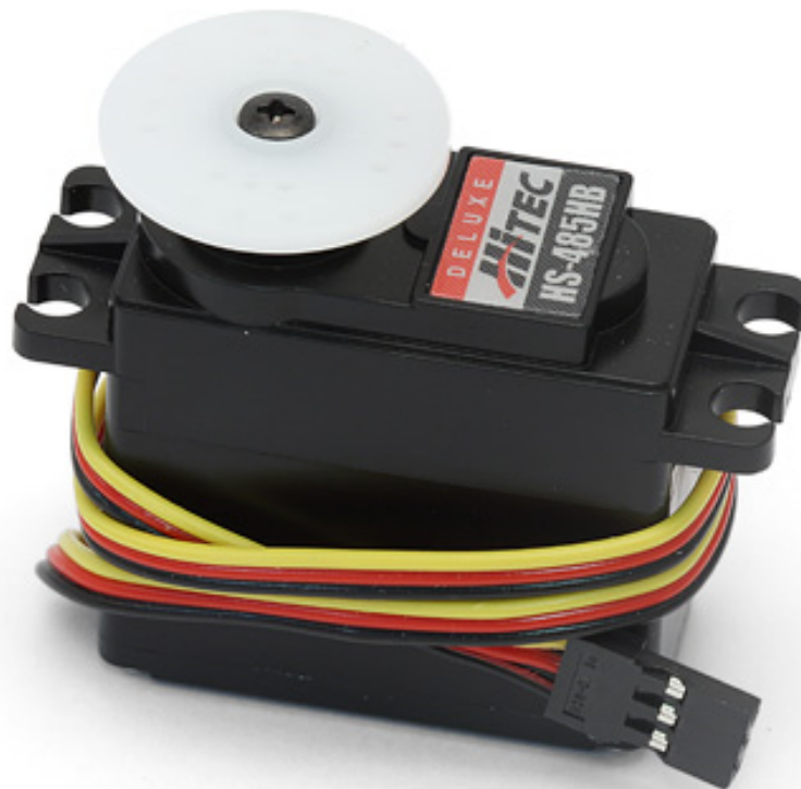
Figure 3: A Hitech HS-485 HB servo. The white plastic mounting hub was replaced with aluminum hubs specifically designed for the drive wheels used. ( www.servocity.com )
