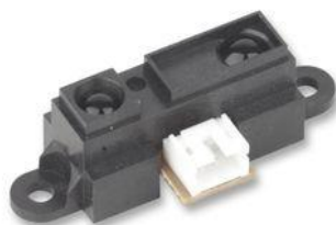
Figure 6 GP2Y0A21YK0F IR Sensor
