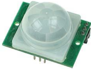
Figure 7 PIR Motion Sensor
