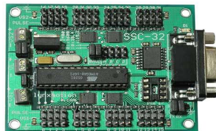
Figure 4 SSC-32 Servo Controller
