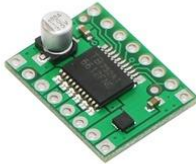
Figure 5: Toshiba TB6612FNG Dual H-Bridge (Image source: www.Pololu.com )
