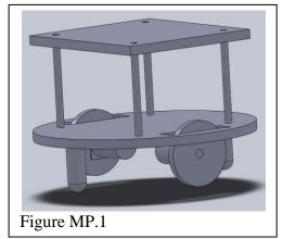
The base platform is circular in shape, with 2 cutouts for wheels. The circular shape prevents the robot from getting stuck in case of collisions. It also provides maximum maneuverability, enabling the robot to rotate in place. Half
