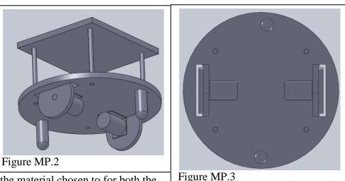
inch thick plywood was the material chosen to for both the bottom and top level. It provides exceptional strength,
