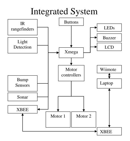
The Epiphany DIY board is the base of this robot. It accepts input from the IR range finders, sonar range finder, and the CDS cell. GPIO pins are used to accept input from the buttons and Bump sensors. GPIO pins are also used to control the the LEDs, LCD, and buzzer. The motor driver integrated into the Epiphany board is used to directly power two DC motors.
