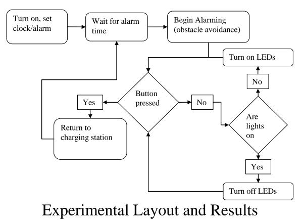
The experiment provided a simulation of the robots intended purpose. The robot and its charging station were placed in an enclosed space (to simulate a room). The robot was then programmed to go off at a certain time. At the time, the robot began alarming and obstacle avoiding. After a minute or so of successfully moving randomly without hitting any obstacles, the large red button on the top of the robot was hit, causing it to seek its base station.
