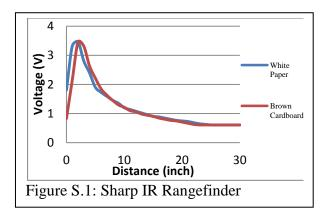
measured by the Epiphany DIY board and the hex result was printed out to the LCD. The hex values were then converted to voltages and the results are in figure S.1.
