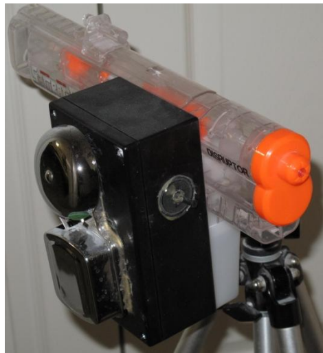
Figure 3: Sound activated squirt gun.
