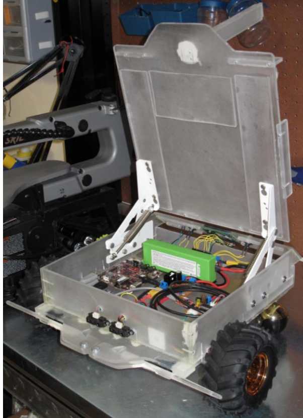
Figure 7: The spring loaded hinges made troubleshooting easier.
