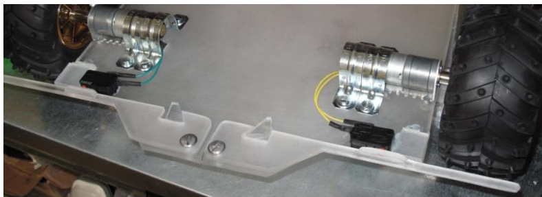
Figure 8: Bump sensors in contact with the bump “paddles” underneath the Buggy.
