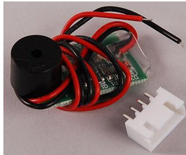
Fig. 12 3S Battery Monitor
