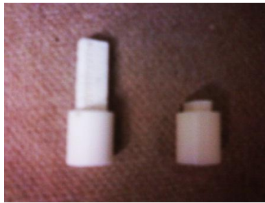
Fig. 3 On the left is a wheel adapter is still intact and on the right is one that has failed in shear
