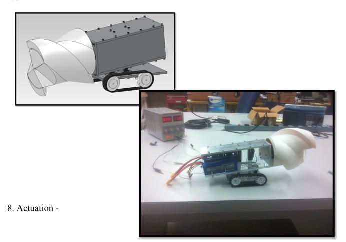
The actuators on the robot are two linear actuators, two micro geared motors, and a larger geared motor. The two linear actuators angle the drill, the micro geared motors drive the robot, and the large geared motor spins the drill bit.
