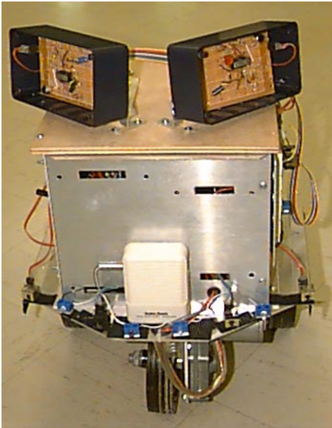
Figure 3: Autonomous agent (front view) showing IR emitter/detector pairs, ear sensors(blue boxes), and speaker(white box).
