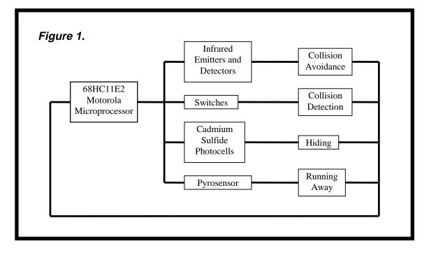
The diagram shows that there is a different type of sensor for each behavior the robot exhibits. All the sensors are controlled by the microprocessor and the behaviors are determined by the programs written in C.
