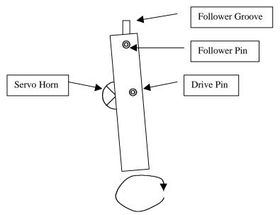
With this simple leg design I am able to make Sparky walk forward and backward, turn left and right. However, since I am not able to center his center-of-gravity over three legs before I move the fourth, a method of dynamic stability is required. For this, I chose to use a 1-2 Gait and balance Sparky on two legs for half of each step cycle.
