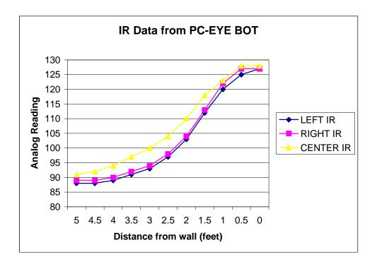
It can be seen that the distance vs. IR values is fairly linear over a range from about 4 feet to 0.5 feet away from the wall.
