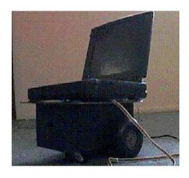
The laptop is connected to the 68HC11 through a serial connection to the communication board that provides for translation from RS232 values to TTL levels.
