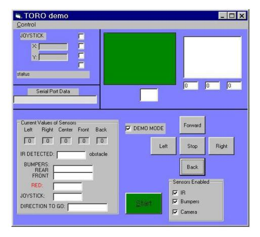
As can be seen this program shows everything that is occurring with all of the sensors so it is very easy to see what is happening and correct it in real-time. The only necessary tests that were conducted were for performance. The overall performance of this application in controlling and & communicating with the robot is found by running the control loop 50 times and timing its duration.
