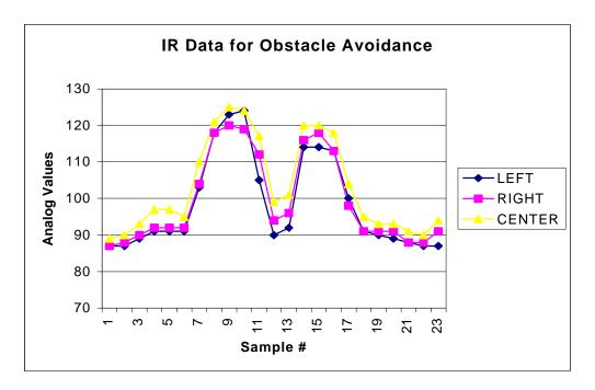
Here the first bump shows an obstacle on the left and the second shown an obstacle right.
