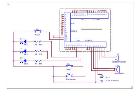
The two figures below show the pin-out of the sensor and the schematic.
