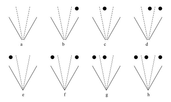
Using these 8 possible scenarios and the concept of fuzzy logic, the uController will determine which direction to head towards. The range of detection for the pir sensor is from \$0E to \$21 providing the following boundaries. Using the values on the left of the table below to produce values for the clockwise and counter-clockwise detection. It is placed into the table on the right to provide a fuzzy logic response to determine the direction to head towards.
