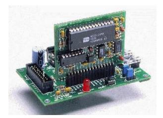
The module itself is interfaced with the Atmel chip through serial communications. The first step is to initialize the sound chip, i.e. Setting the playback mode and volume level on the amplifier. After this has been done all you have to do is send the byte code for the sound clip that you want to play.
