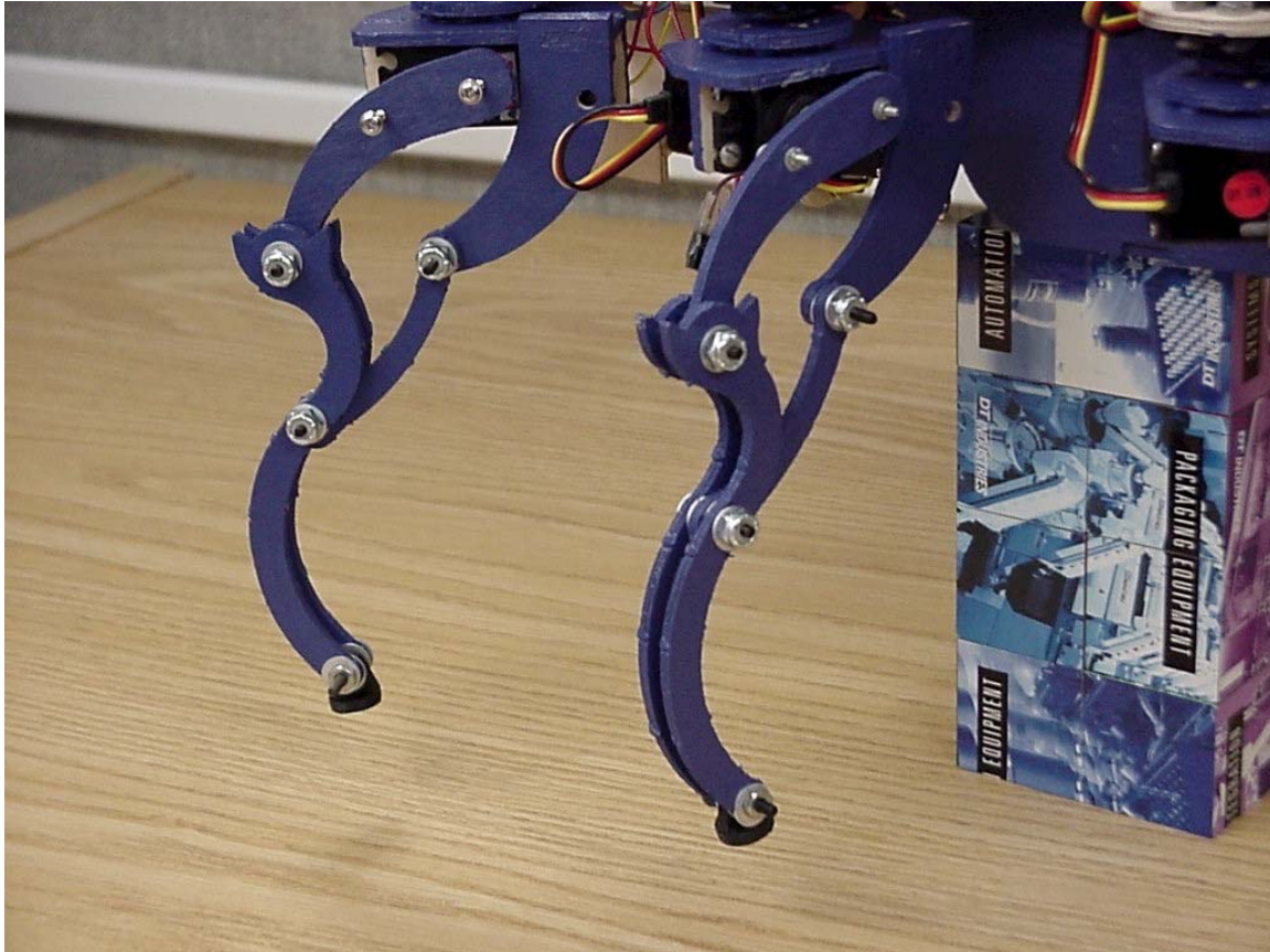
Figure 9. Photograph of physical legs after they were finally constructed, assembled, and painted
