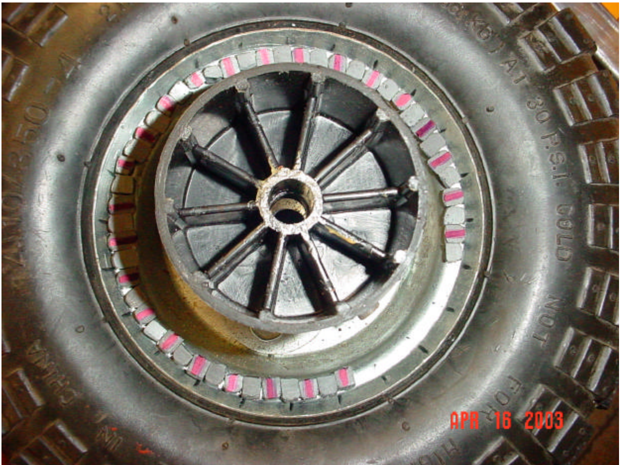
Figure 5: Mounting the magnets on the right wheel for the Hall effect IC.
