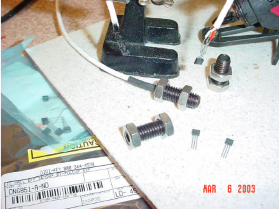
Figure 4: The process of mounting the DN6851 Hall effect IC.
