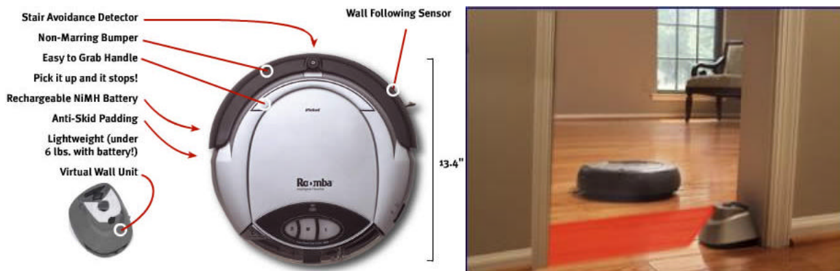
Figure 1: Roomba's anatomy on left and in motion on right utilizing its virtual wall unit to close off adjoining rooms.
