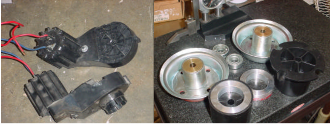
Figure 5: Motors on left and machined bearings, sleeve, and housing on right.
