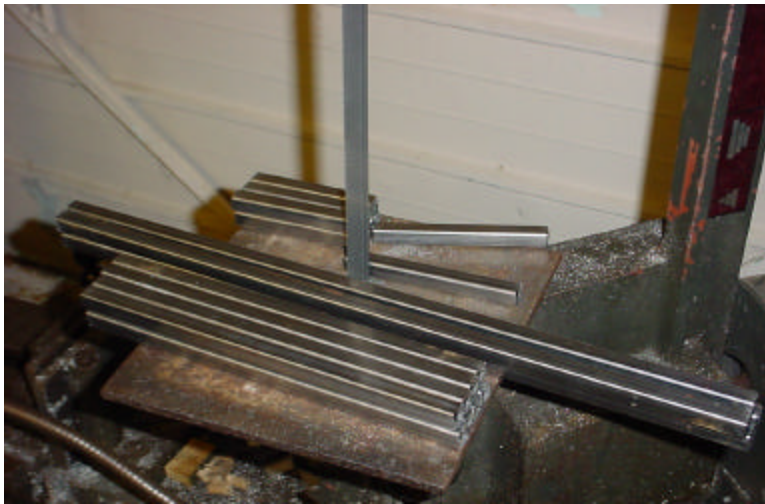
Figure 4: Square steel to be used for platform.
