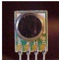
Figure 5. TWS-434A RF Transmitter Module
