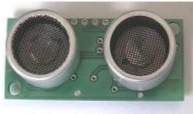
Figure 1.Devantech SRF04 Ultrasonic Range Finder
