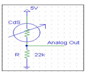
By using this circuit I was able to get accurate readings for each resistor. By taking readings in a well light area for a dark area I was able to compare the value for each photo resistor.
