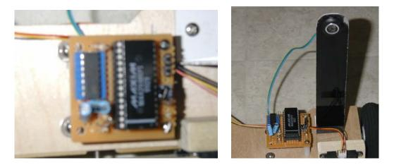
The schematic above was built on one of the PC mount boards that I previously mentioned. I used wire wrap sockets going into the board because they are easy to work with when wiring and soldering. Once again, this is very time consuming especially when you must build three of them. As you can see in the picture, I mounted the board on my platform right next to the stand that holds the sonar transducer.
