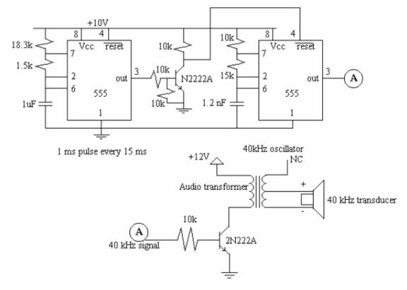
The 555 timer on the left produces a 1 ms pulse every 15 ms. The 1 ms pulse is a 40 kHz signal being transmitted out a transducer. This 40 kHz oscillation is being produced from the 555 timer on the right.
