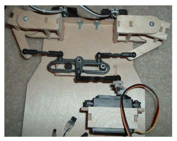
With the robot completely done, and steering tried and true, I would say that there are some bugs to be worked out. The steering system is limited by a few factors on my robot. In the picture above you can see that the steering is almost at it maximum right turn, but if you notice the servo is nowhere near it's maximum. The max right hand turn
