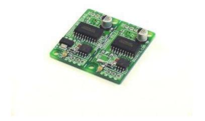
The motor controller that was used it the Sozbot HB-03. It operates in a voltage range from 6V-18V. It has proven to be a well built component that can handle a peak current of 5 amps. The controller is dual channel, bidirectional, and operates on servo style PWM's (or RC style). It was an expensive board, but the reliability and great characteristic made it a worthwhile purchase.
