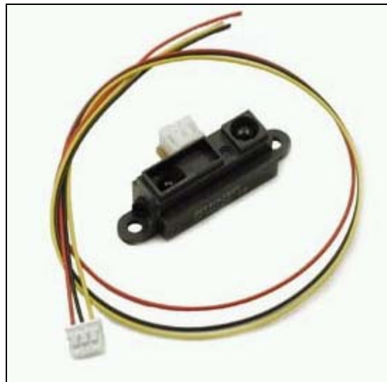
Figure 4: Sharp GP2D12 Detector Package.
