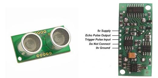
In addition to an array of SRF05 sensors, a Devantech SRF08 sonar range finder will be used for the front of the robot. The SRF08 is the smarter cousin of Devantech's popular SRF04 sonar sensor. It provides twice the sensing range of the SRF04 plus an on-board MCU which handles the critical timing functions and distance
