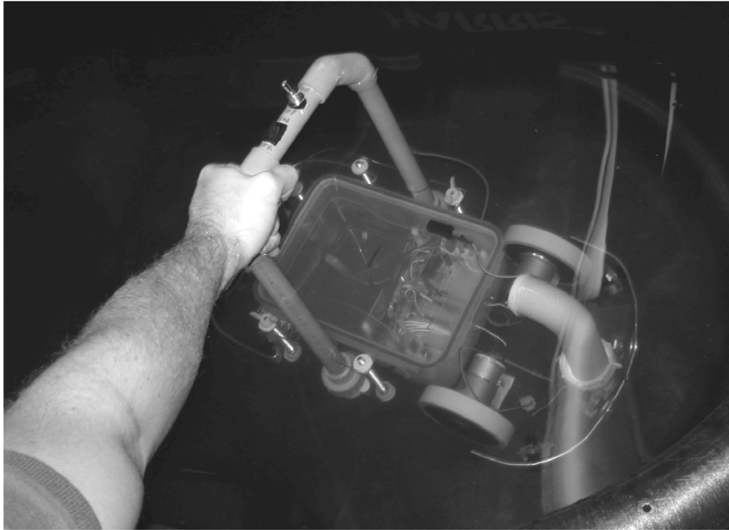
Figure 17. Initial underwater test of the robot
