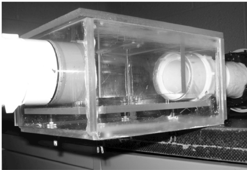
Figure 11. Side front view of the sensor plate in the payload bin
