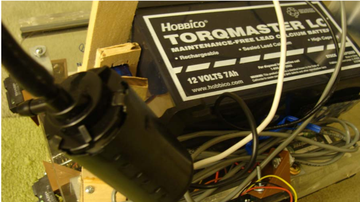
Figure 2 - The windshield washer pump is powered by a gigantic and heavy 12 V, 7 Ah battery. The battery was inexpensive and worked well for my platform.
