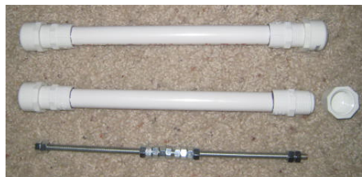
Figure 6. System for Buoyancy Fine Tuning and Center of Gravity Adjustment.
