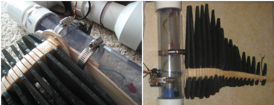
Figure 8. Wing Internal Frame with Angle of Attack Adjustment and Servo Actuator.
