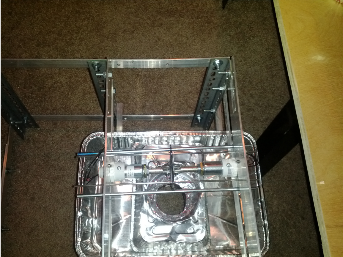
Figure 6: Egg Cracking Subsystem with Linear Solenoids
