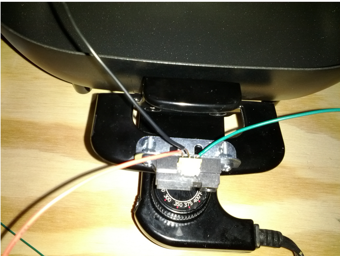
Figure 8: IR Sensor attached to handle of Electric Skillet
