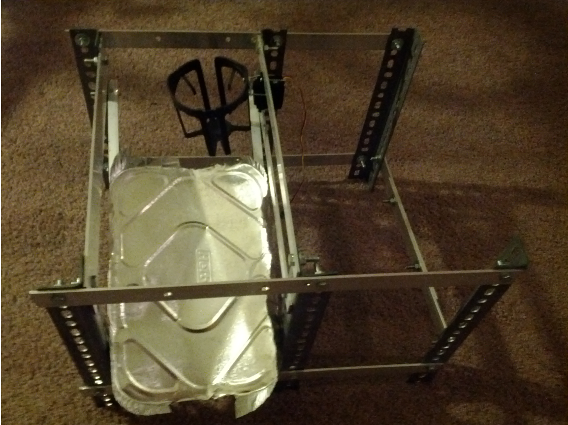
Figure 7: Egg Pouring Station with High Torque Servomotor
