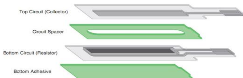
Figure 10: Membrane Potentiometer (Layers)
