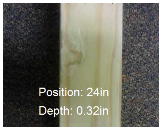
Figure 23: Sample image of Android capture and position and depth superimposed onto image using MATLAB
