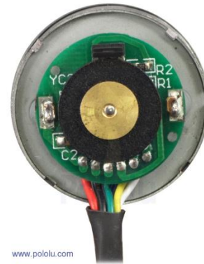
Figure 20: 64 CPR Encoder Mounted on Motor 1
