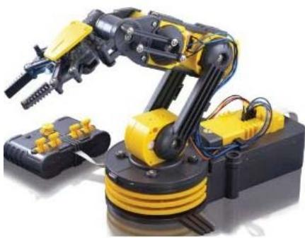
The robot arm, consists 5 motors, use arduino and motor driver circuit to control it.
