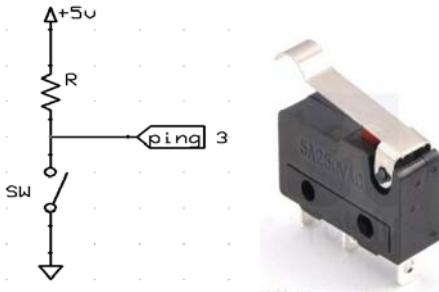
When touch sensor been touched, the arduino will receive a high signal, but to eliminate the noise, I use delay(50); to check the bump switch is actually been touch.
