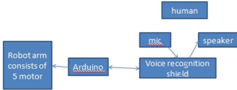
The voice recognition shield can interface with human, and use arduino to control the robot arm.
