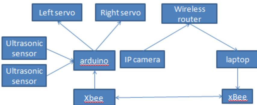
Two Ultrasonic Sensors can help the arduino know the distances in the front. The arduino can provide different plus wild to control the servo. Base on these components , the robot can do obstacle avoidance.
