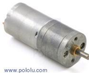
Figure 7: 75:1 Metal Gearmotor 25Dx54L mm, Key specs at 6 V: 75 RPM and 80 mA free-run, 85 oz-in (6.1 kg-cm) and 2.2 A stall.
