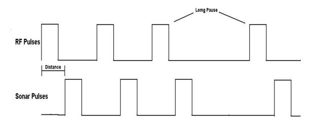
By calculating the time it takes between receiving the RF pulse and receiving the sonar pulse one can determine the distance away from that beacon. The actual design that was used for the controller circuit will be discussed in the sensor section.
