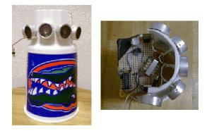
The functional layout for the controller is relatively simple. The three beacons emit a single pulse in the same sequence followed by a long pulse after the third beacon. This pause helps determine which beacon is the first beacon. At the same time each beacon pulses, a RF pulse is also released.
