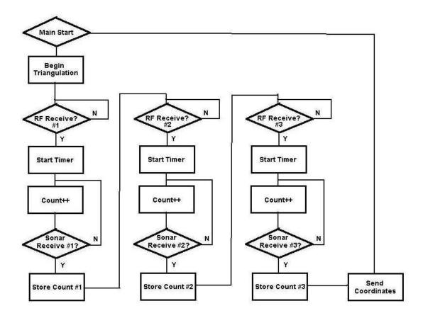
This software works correctly as shown and even transmits the coordinates on HyperTerminal. The coordinates are sent through a different frequency RF to a computer connected to the receiving RF board.
