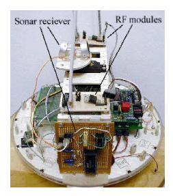
The receiving end will first look for the three-pulse sequence in order to identify the first pulse. Next it will start timing loops in order to determine the distance from the beacons.
