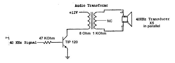
We had to turn this circuit on and off frequently because of the way it was acting. Once on the signal would start at about 15 volts peak to peak. Then the longer it was on the signal would grow continuously. The TIP120 would get very hot (hence letting more voltage through) and the transformer would burn. This is why we chose to hook the
