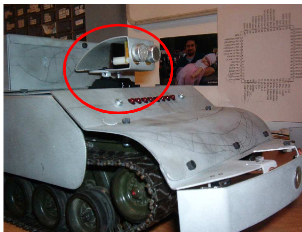
Figure 3. SRF08 Mounting Location
