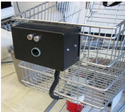
Figure 6 Vision and Sonar implementation
