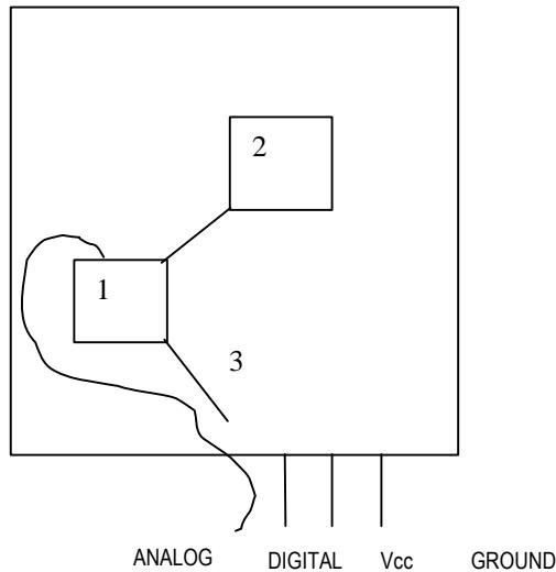
Basically, trace 3 above was cut and a wire was soldered to the top of box 1 which is a  $0.1\mu F$  capacitor to have access to analog readings from the IR receivers. Box 2 is the integrated section.
