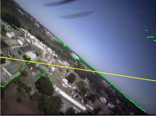
Fig. 2: An early attempt at horizon detection. Pixels marked in green indicate the sharpest distinction in color values down vertical columns; the yellow line indicates the consequent incorrect horizon detection.
