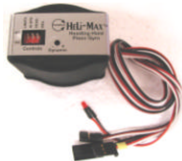
Figure 15 – Heading Hold Piezo Gyro
