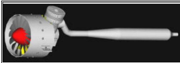
Figure 08 – Dynamax Fan and O.S. Max .77 engine
