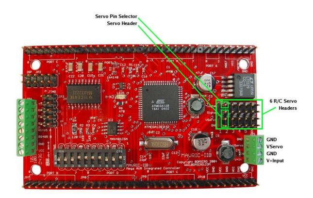
Each of the 6 servo connectors is composed of 4 pins as shown. The bottom three pins are labeled Signal, VServo, and GND and is where the servo connector is connected. The 4<sup>th</sup> pin located above the servo connector and labeled Signal on the MAVRIC-IIB silkscreen and *Servo Pin Selector* in the diagram above is used to select which ATmega128 pin is used to drive that servo. This layout was chosen because most of the ATmega128's available I/O
