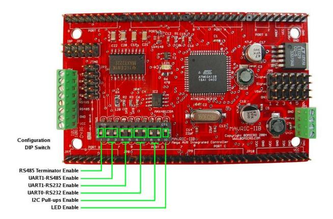
Note that the UART1 RS485 and RS232 selection DIP switches must not be in the "ON" position at the same time. When change the configuration of the UART1 selection, always turn off UART1-RS485 and UART1-RS232 first, then turn on either UART1-RS485 to enable the RS485 interface, or turn on positions UART1-RS232 to enable the RS232 interface. Never turn on both UART1-RS485 and UART1-RS232 simultaneously. See the following table for the settings.
