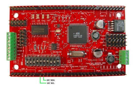
Note that in order to utilize these pins for  $I^2C$ , the  $I^2C$  pull-ups must be enabled (DIP switch positions 8 & 9 ON), and the  $I^2C$  interface must be enabled by your firmware program.
