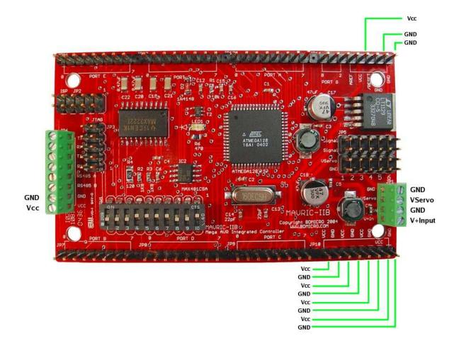
Note that all **VCC** connections are regulated 5.0 Volts, input or output. Connections labeled V+ are unregulated 5.5 - 15V input and feed into the on-board regulator where it is regulated down to 5 Volts for the board electronics. The Vservo connection point powers only the 6 servo headers and should be limited to the range of 4.8V - 6V. Some servos can handle a higher voltage, but double check your servo specs before applying a higher voltage.
