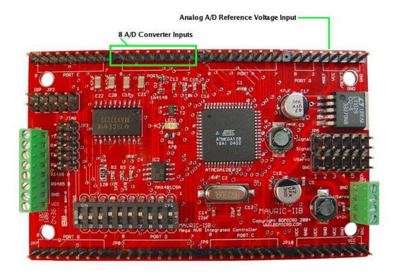
The on-board voltage reference of the ATmega128 remains available and can be configured to match either Vcc (5.0V) or set to 2.56V by setting the appropriate bits of the ATmega128's ADMUX register. Note that while the external A/D reference pin is provided, the on-board reference is sufficient for many applications.
