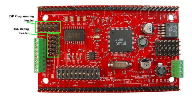
Both headers can be used to download the firmware to the MAVRIC-IIB board. The JTAG header, in addition, can be used to provide source level single-step debugging of your program as it runs natively on the chip itself. The JTAGICE or equivalent programmer is required to utilize the JTAG header.
