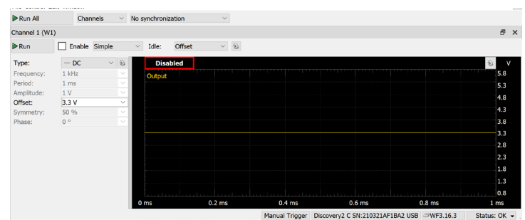
Figure 28: Using Wavegen to Make a DC Voltage
